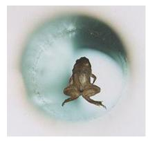
A live frog levitates inside a 32 mm diameter vertical bore of a Bitter solenoid in a magnetic field of about 16 teslas at the Nijmegen High Field Magnet Laboratory.
